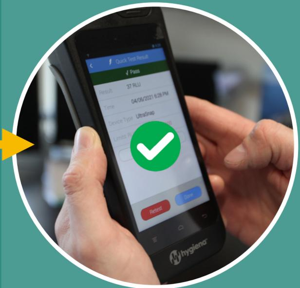
**CERTIFICATION** with **NSPECT™** luminometer to confirm the job is done properly and all targeted areas are effectively sanitized.
